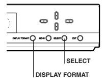
The HDTV Receiver provides several display formats. The DISPLAY FOR-MAT button on the front panel changes the output connector and resolution. The output resolution may be converted from the original broadcast format.
